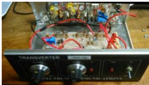
Fig 11 Photograph showing the transverter board on the box base and the PA board on the back.
