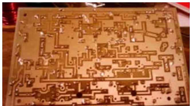
Fig 6: showing etched copper underside of the PCB
